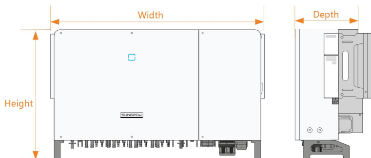
figure 2-2 Dimensions of the Inverter
